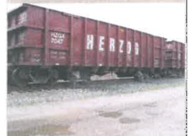
Automatic ballast unloading by Herzog rail car
