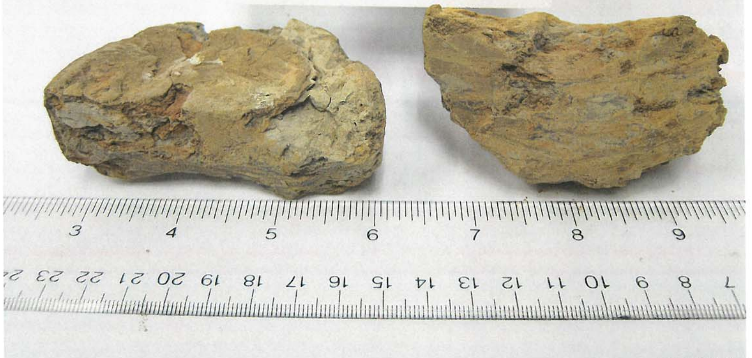
Borehole MP-2 Interval 16 - 17 feet Laminated silt and clay layers
