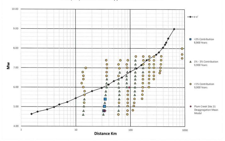
Data from: <a href="http://earthquake.usgs.gov/hozards/apps">http://earthquake.usgs.gov/hozards/apps</a>, e-e' curve plotted from Magnitude-Distance Relations for Liquefaction in Soil from Earthquakes, Bulletin of the Seismological Society of America, Vol. 83, June 1993. % contribution data from txt PSHA Deaggregation parameters - 1% in 200 years, Return Period 9,900 years, Exceedance PGA >/= 0.07774, Annual Exceedance Rate 1.0 x 10-4
