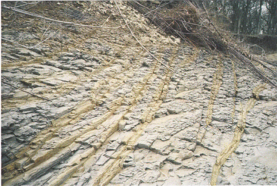
Exhibit TJFA 424-A, Joint Set in Weathered Taylor Marl – Skyline MSW Landfill
