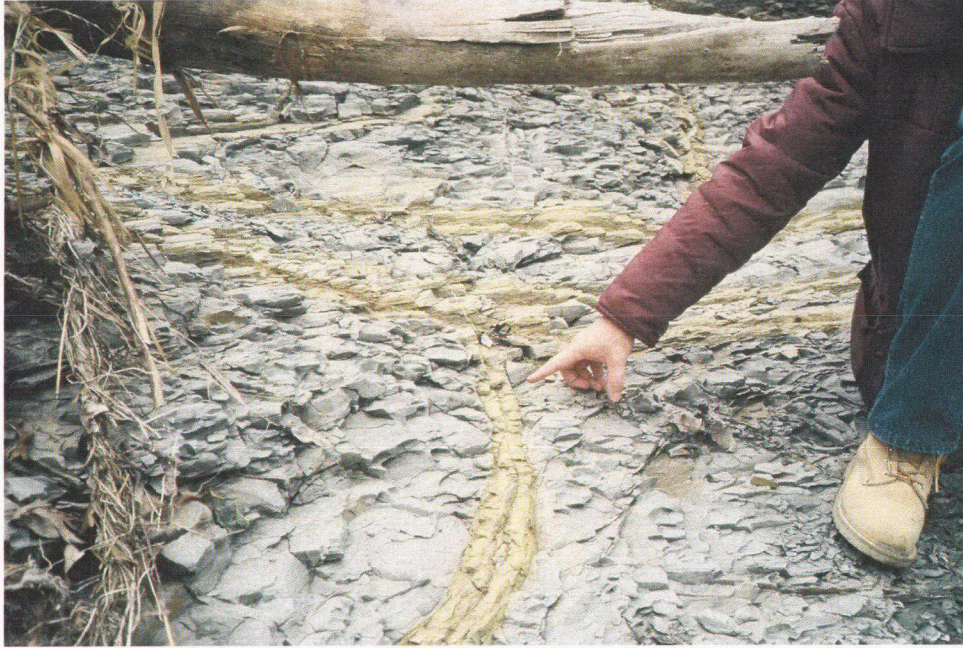
Exhibit TJFA 424-C, Intersecting Joints in Weathered Taylor Marl – Skyline MSW Landfill
