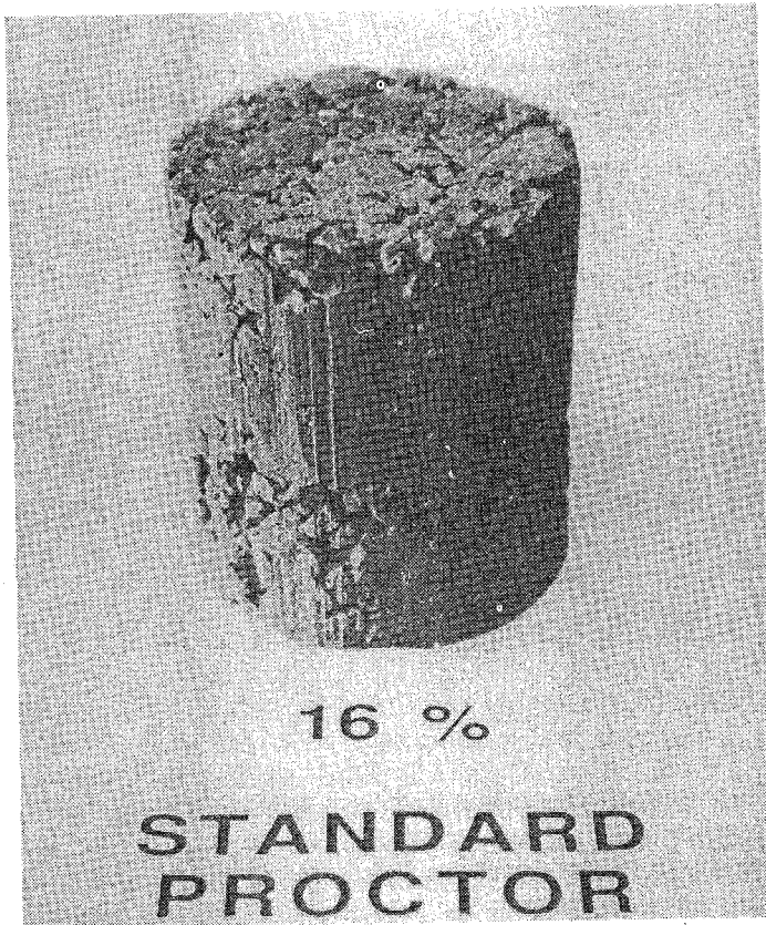
Figure 2-6. Highly plastic soil compacted with standard Proctor procedures at a water content of 16%.
